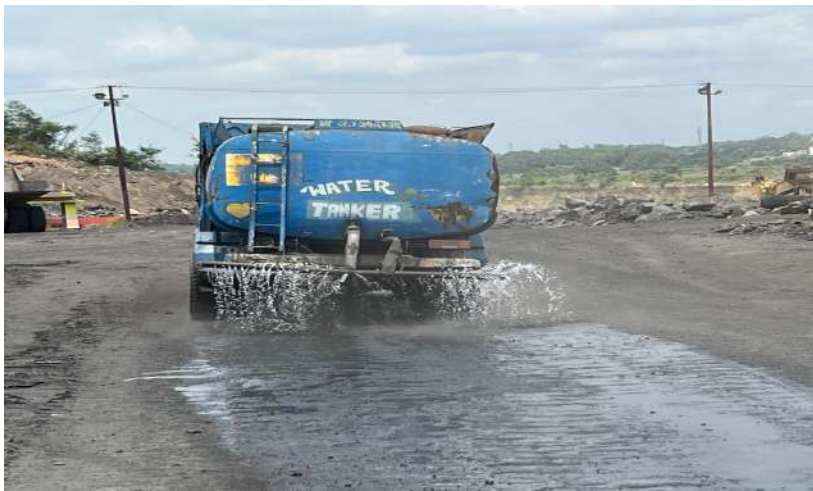
Water Tanker for Sprinkling
