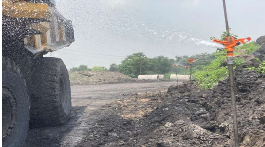
Fixed Type Sprinkler in Open cast mine.
