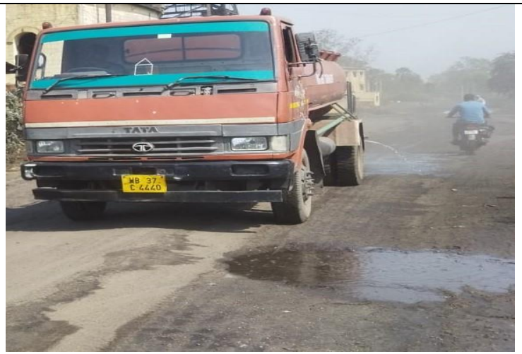
Water Sprinkling at Bejdih Colliery by Mobile Water Tanker.
