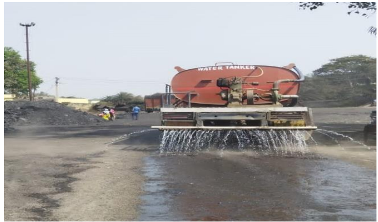
Water Sprinkling at Patmohana Colliery by Mobile Water Tanker.
