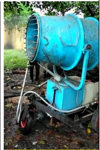
Picture 3: Trolley Mounted Mist Canon at JK Nagar Railway Siding
