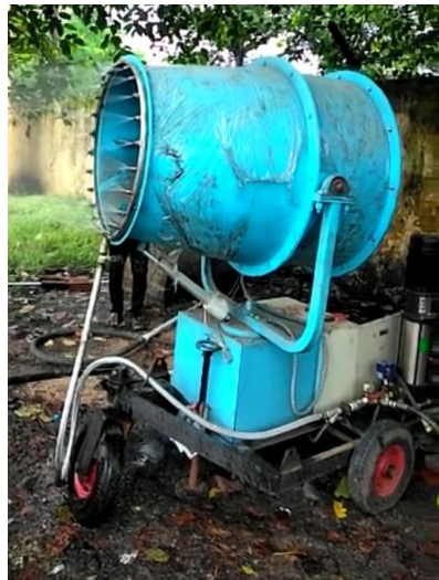
Mist Canon at JK Nagar Railway Siding; Fixed and Mobile Type Mist Sprayer at Modern Satgram or JK Nagar Railway Siding
