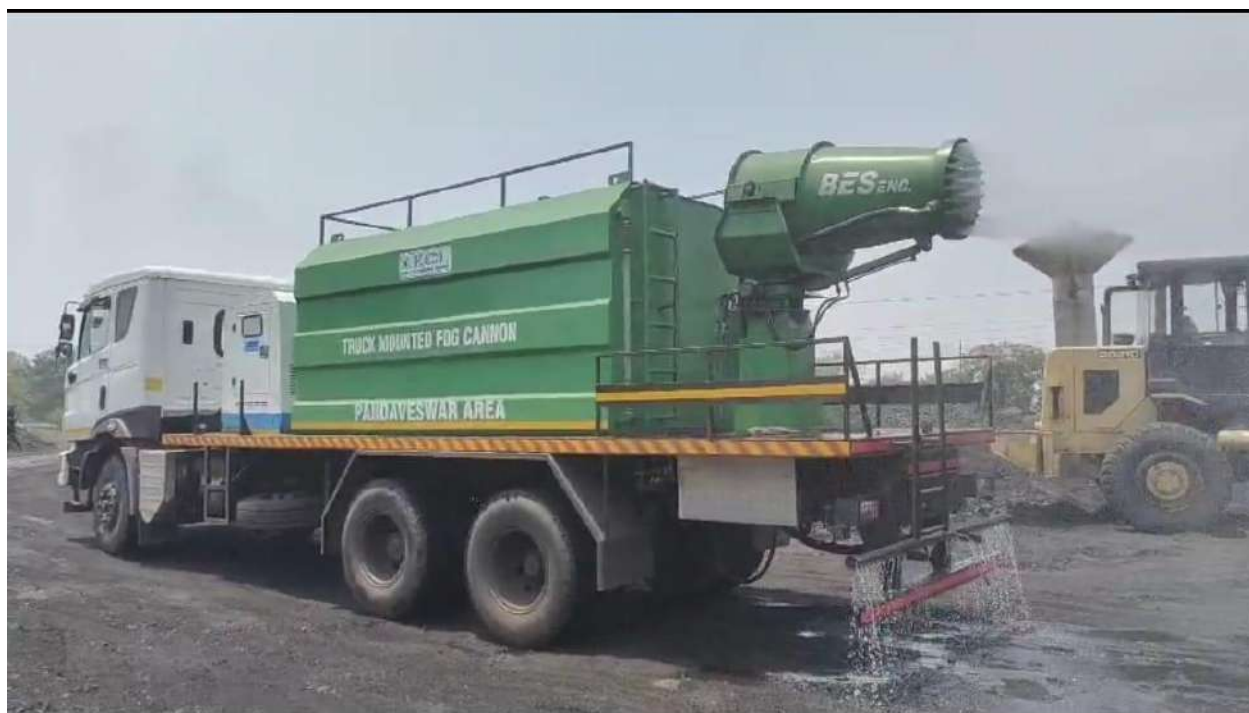
Photograph of recently procured truck mounted fog cannon dust suppression system in operation at S.S. Railway Siding under Khottadih OCP, Pandaveswar Area.
