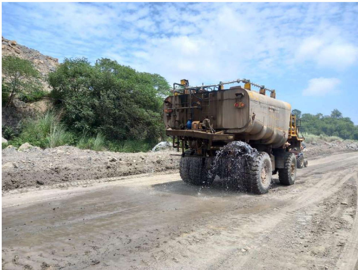
Photograph of dust suppression by mobile sprinkler over the haul road of Khottadih OCP.
